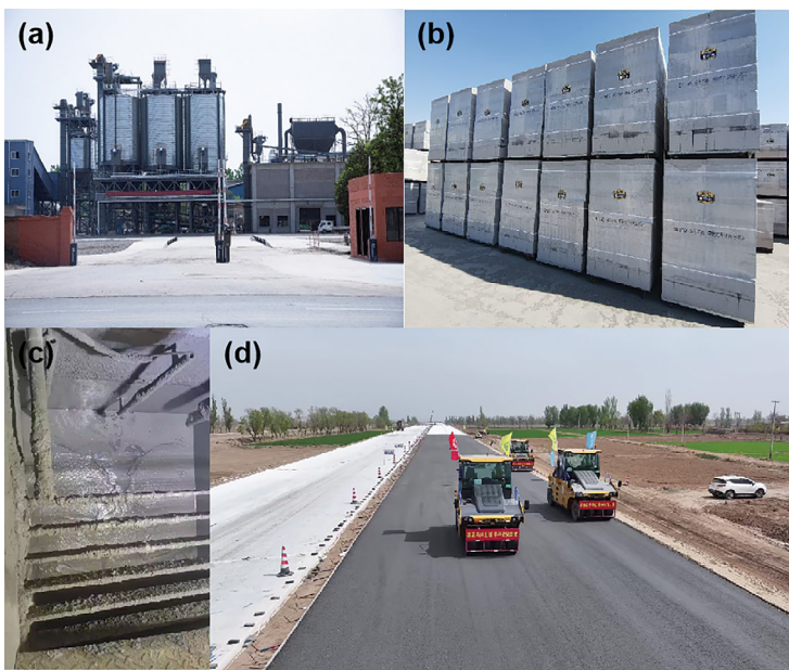
Figure 7 Chemico-activated cementitious materials production and application in China: (a) Geopoly company's plant (1 Mt/year) focuses on one-part geopolymer in Henan Province; (b) aerated concrete production in Shandong Province; (c) mining backfilling in Shanxi Province; (d) road base construction in Ningxia Province. Photos courtesy of Geopoly company
