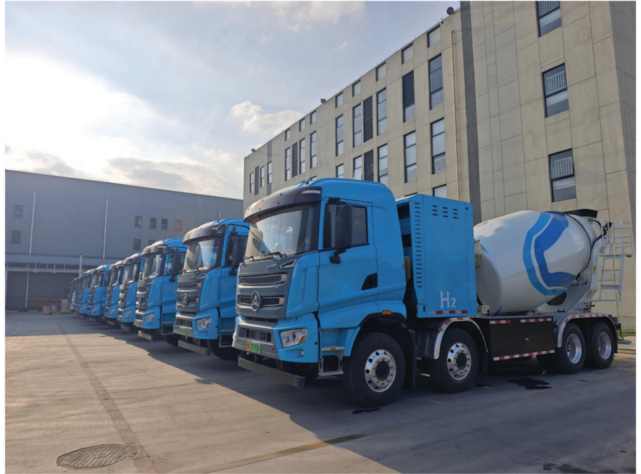
Figure 1 Hydrogen-fueled concrete transport tankers promote the low-carbonization of logistics and transportation
