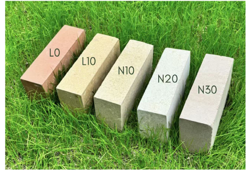
Figure 2 Range of earth4Earth bricks with standard UK size (215 mm × 102.5 mm × 65 mm). L0 Brick: no e4E lime and is a low-carbon brick and can be used in projects where traditional raw earth techniques such as adobe are envisaged. L10 Brick: Contains 10% conventional/commercial hydrated lime as binder. L10 has a significantly reduced carbon footprint compared to a traditional fired clay brick and sequesters CO 2 during use. N10 Brick: Contains 10% of e4E zero-carbon lime binder. Because the binder is made without releasing CO 2 , the N10 brick is carbon-negative over its life cycle and it absorbs a total of ~0.18 kg CO 2 from air per unit which exceeds any remaining emissions. This model has been third-party verified as carbon-negative via an EPD. Its mechanical compressive strength can reach compressive strengths up to 40 MPa (observed, not declared). N20 Brick: Contains 20% e4E zero-carbon lime binder. With double the binder, it achieves double the CO 2 uptake capacity. These units can capture ~0.35 kg CO 2 each over their service life. N20 bricks show increased carbon sequestration due to the higher binder content. N30 Brick: Contains 30% e4E zero-carbon lime binder. This high binder fraction maximizes carbon capture. Each N30 brick locks away ~0.5 kg of CO 2 over its lifetime, turning a brick into a half-kilogram CO 2 storage unit. N30 represents the premium carbon-negative product with the greatest climate impact per brick. This performance has been independently verified through a third-party Environmental Product Declaration (EPD)
