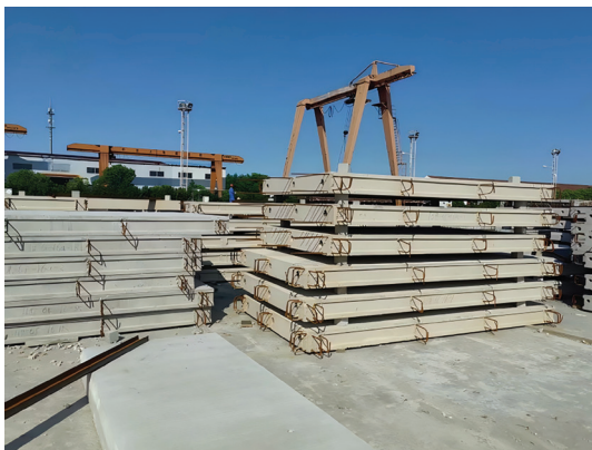
6 Outdoor ageing of precast ribbed wall panels
