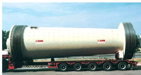
3 TCM 3.7 / 2.45 x 17.5 m tube cone mill
