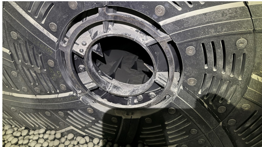
1 Installed Christians Pfeiffer's Open Lifter Diaphragm for GGBFS processing
