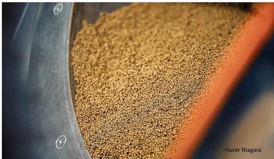
4 Limestone pellets with ideal grain size distribution
