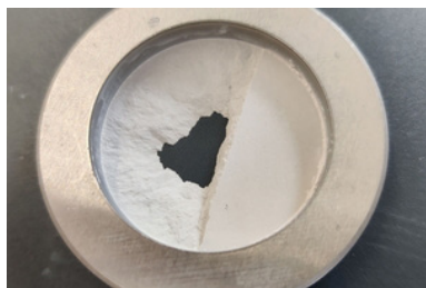
4 Lower surface of a pressed tablet first broken by lamination after incomplete de-aeration during pressing and eroded by compressed air
