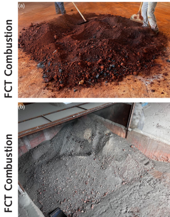
5 FCT/Cemaxx Pilot Plant, (a) raw, and (b) calcined clay with IM
