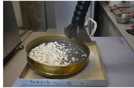
1 Crushed, screened and prepared gypsum mould breakage for thermal activation
