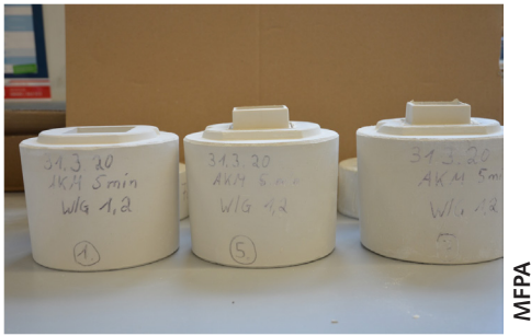
3 Standard mould made of RC plaster
