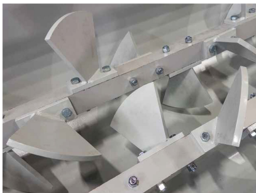
10 Mixing paddles in a lime hydrator
